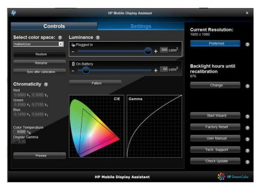
The DreamColor display was not only less expensive than the cathode ray monitors it replaced, but it doesn't need to be color calibrated for at least 1,000 hours. This backlit LCD display has a resolution of 1920 x 1200 pixels, features over one billion colors and a wide  $172^{\circ}$  viewing angle.
